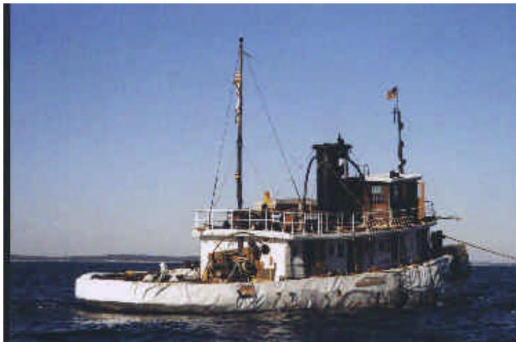
*A view of the LUNA off Manchester, MA. The Sarnafill hull wrap that kept her afloat for five and a half years is remarkably clean. A scupper can be seen cut through the aft bulwark. Two generators are located on the boat deck aft. A Zodiac raft is located on the stern deck and a skiff is located on the boat deck. The guy wires running from the top of the funnel can be seen.*
